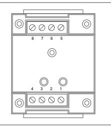
The Signature Series Dual Input Module (model GSA-CT2) is an analog addressable device used to connect one or two Class B, normally open, alarm, supervisory, or monitor type dry contact initiating device circuits (IDCs) to a Signature loop controller. Two device addresses are required.
